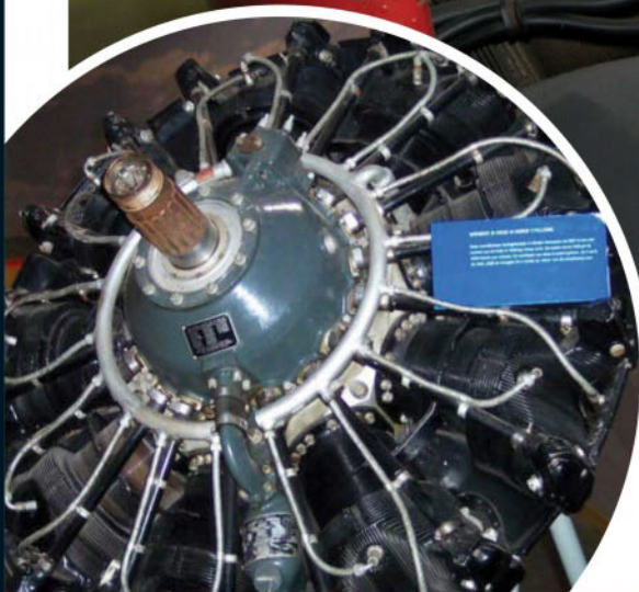
Left: B-17s were equipped with reliable Wright R-1820 Cyclone radial air-cooled engines. First produced in 1931, these engines remained in production until the 1950s
